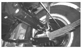
the spring plates and shock absorbers, check straps disconnected from the axle, rear spring shackles removed - and bingo all done.
