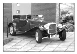
First registered 2007 - Donor 1978 Rubber bumper MGB-GT -Engine professionally reconditioned, new big ends, main bearings, oil seals, water pump. Unleaded head.
