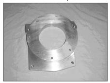
Figure 7 - Completed adapter plate
