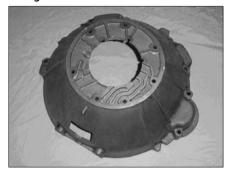
Figure 6 - Bored out auto bellhousing
