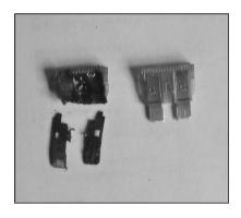
quite warm on high speed especially having liitle cooling in a rubber enclosure. I guess that over time the fuse/holder contacts have heated up enough to start to oxidise, thus increasing the contact resistance and thus increasing the heating effect still further. Setting in train a vicious circle until failure. Solution ? - run separate feeds to the two speed fan, each with a 15amp fuse and leave off the weatherproof caps—should do the trick and easy to achieve.
