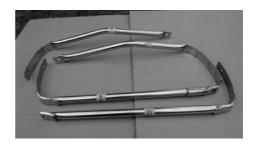
A pair of brand new stainless steel 19" wing stays. I had two pairs made for a NGTA one set for me and one set for my friend who no longer needs them. These have been made to fit the MGB front axle by mounting through the steering rack bolts. These are the tricky items to get the shape right, the rears just mount to the side of the body. They cost £160 a set to have made, **asking £80**
