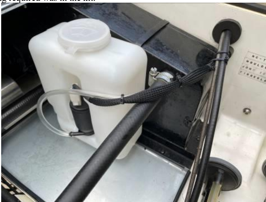
The completed washer bottle installation.
