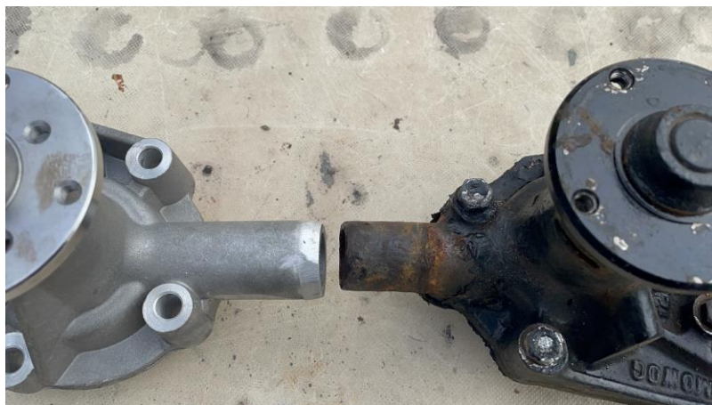
Removing the raised bead enabled the 1-1/8" ID silicone hose to fit over the 1-1/4" OD water pump inlet without undue distortion.
