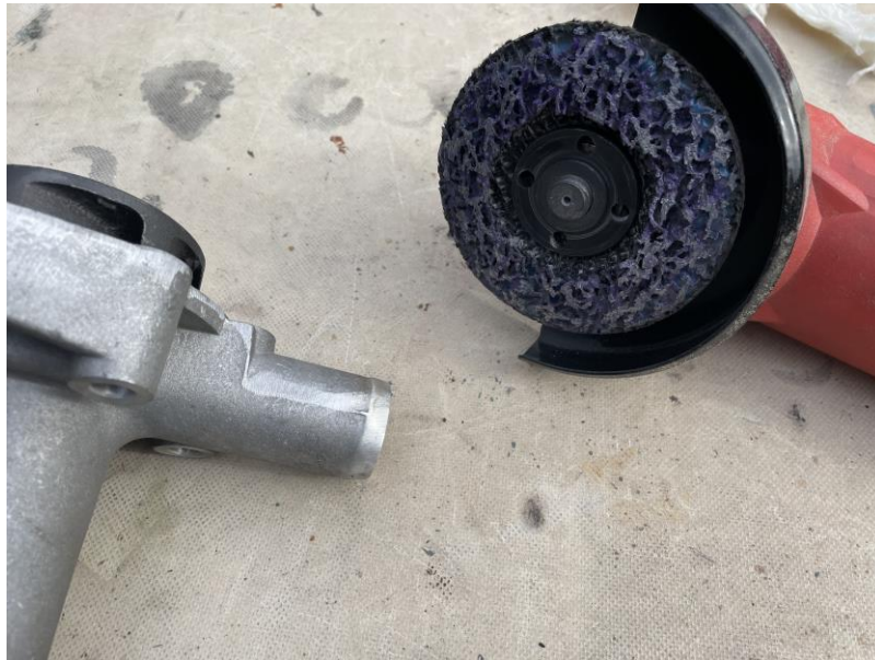
A Polystrip pad in an angle grinder made short work of removing the bead.
