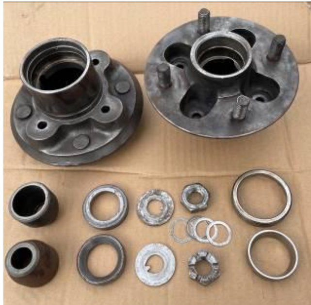
The cleaned and de-rusted parts.
