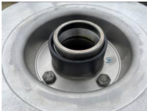
Using the old bearing race as a drift or pressing spacer.
