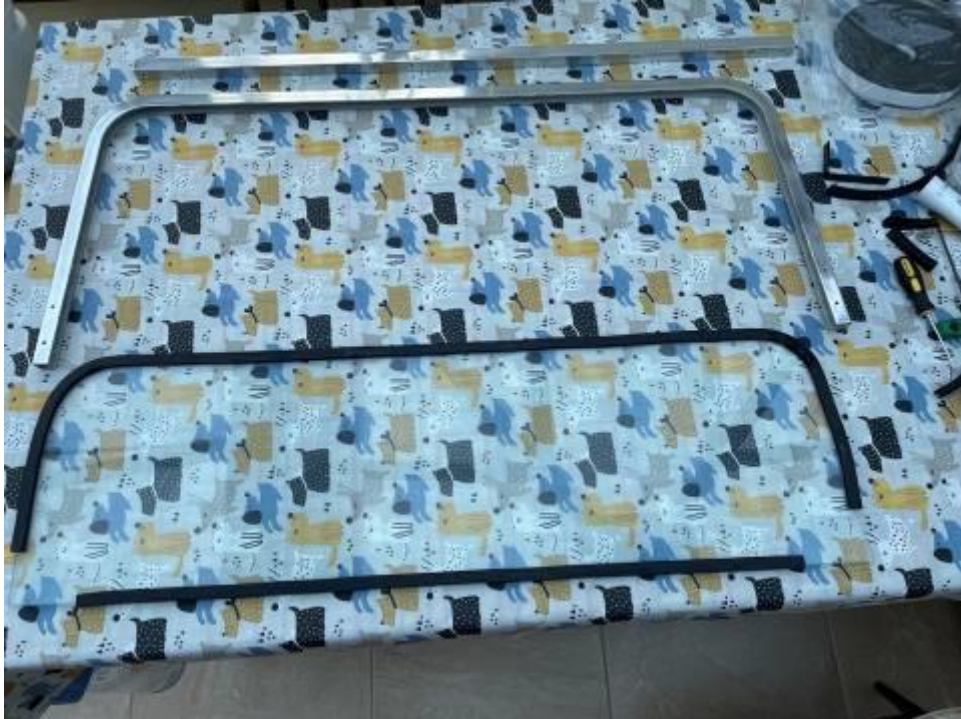
Rubber fitted to glass and ready for assembly, note cut-outs in the rubber for corner brackets.
