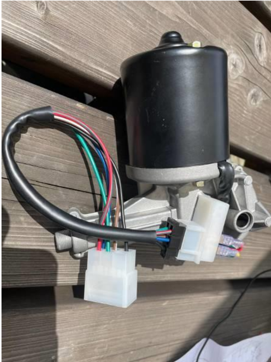
6-way socket fitted.
