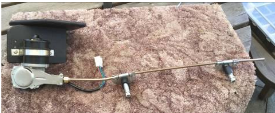
The finished rack assembly ready for fitting, note the angled spacers on the spindles.
