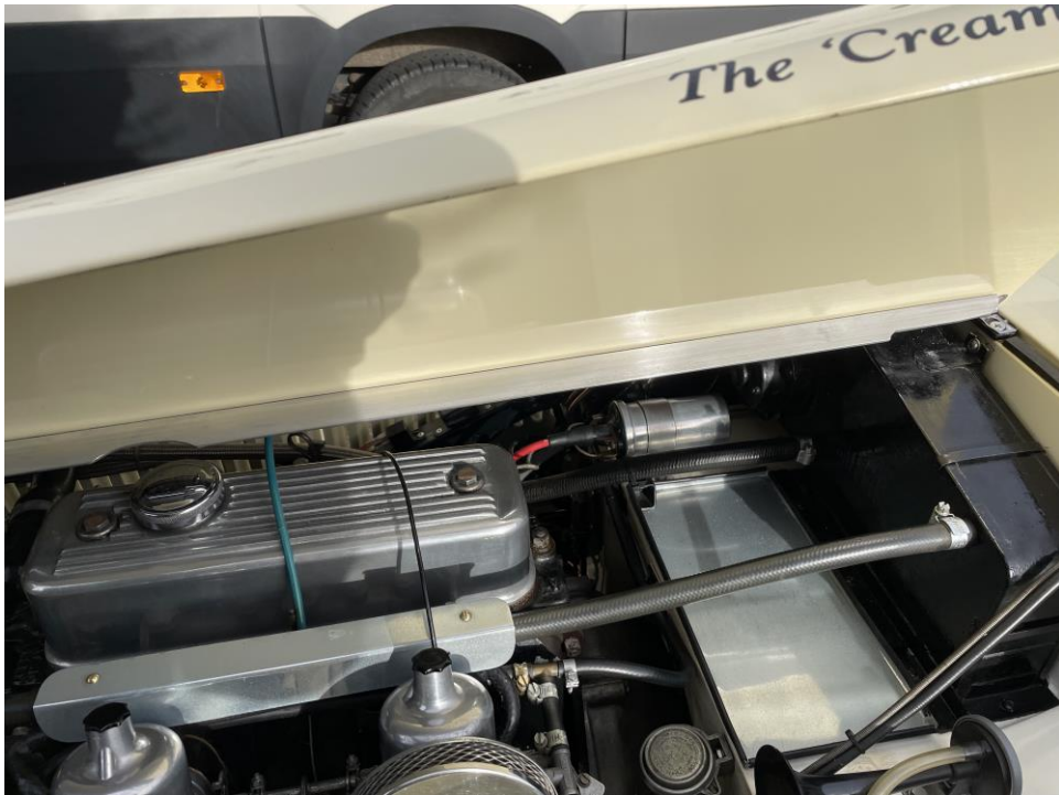
Aluminium equal angle cut of for heater and oil filler cap clearance.
