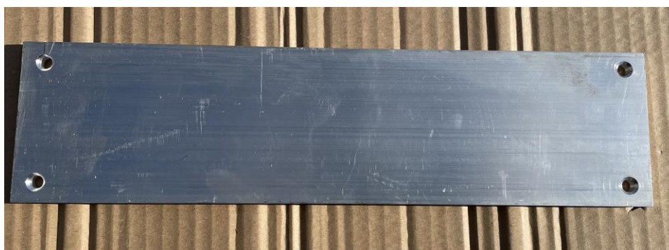
Corner holes drilled to mark edges of seatbelt slot.
