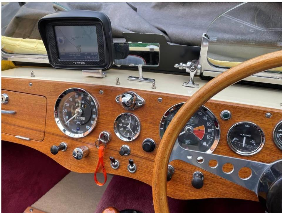
Originally Cracker must have had separate oil pressure and water temperature gauges as there is a newish combined oil/water gauge fitted, with an unserviceable oil pressure gauge filling the spare hole. A voltmeter gauge was purchased to replace the u/s gauge.
