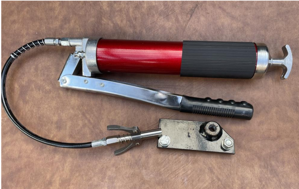
Fitted with the quick release coupler.
